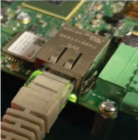
PPR with Active Ethernet Connection
